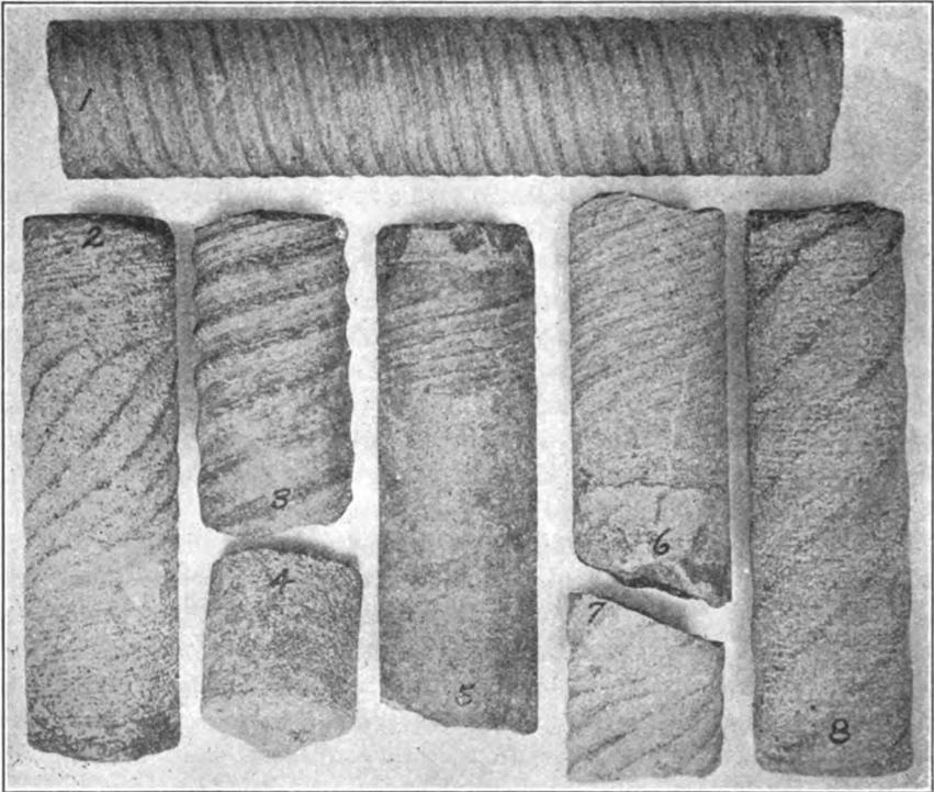
FIG. 1.—SAMPLES OF CORES IN LIMESTONE SHOWING RIFLINGS.
